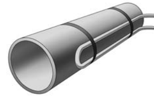
FIG. R - Clamped to walls, hoppers, and pipes
